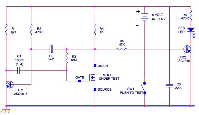
Circuit was recently developed to test N-Channel Mosfets like IRF520, ERF2030.
